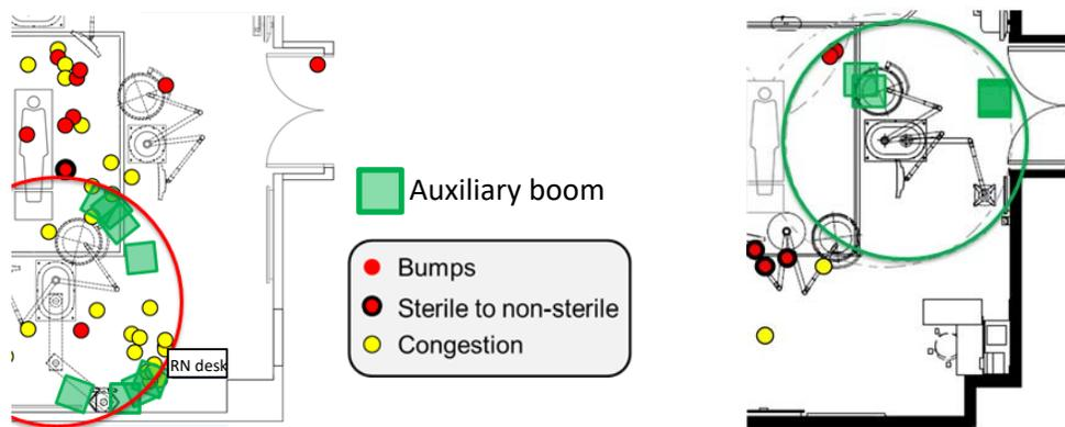
*Figure 6.* Comparison of congestions in the initial mock-up design iteration (left) to the final mock-up design iteration (right) suggested that access to the nursing station was improved; there was less congestion in the space around the nursing station. Furthermore, the potential range of motion of the auxiliary boom in the final mock-up design iteration (green circle), included the full length of the OR table, which was not the case in the initial design (red circle).
