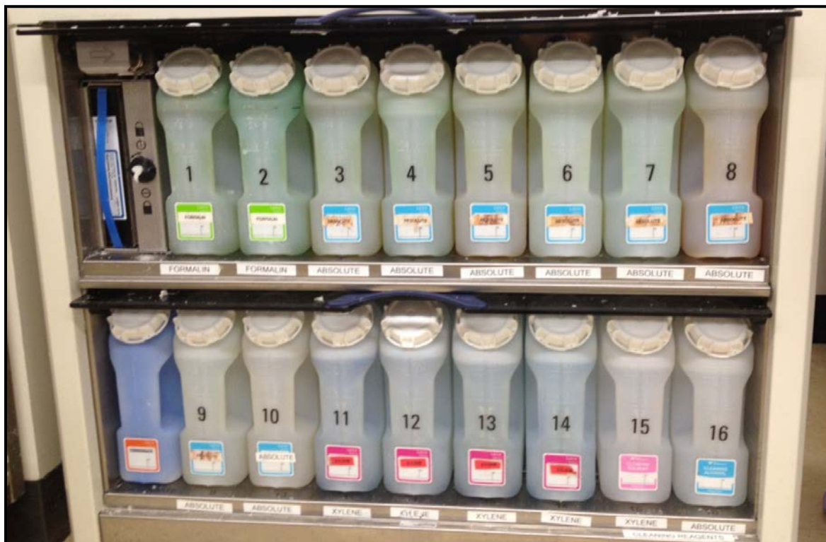
P: Corresponding colour-coded labels on the tissue processing machine reservoirs
